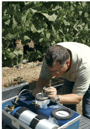
Dr. Mark Greenspan of Advanced Viticulture performs a stem water potential measurement by inserting a leaf petiole into a pressure chamber, cut end up, sealing and pressurizing the chamber, and watching for the first drop of sap to exude from the petiole. (Three Most Common Methods of Measuring Water Status" Practical Winery and Vineyard, Nov/Dec 2006)
