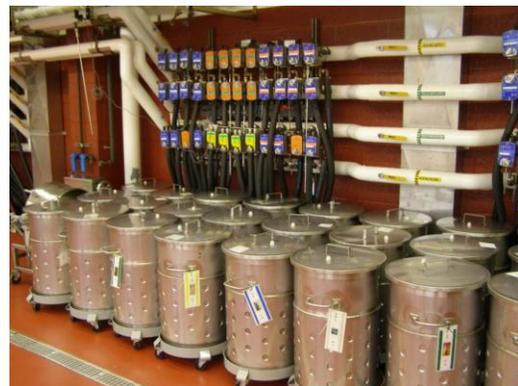
World's smallest temperature controlled stainless steel fermenters
