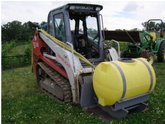
It costs twice as much to develop a hillside as a normal vineyard site, but management costs are a third less because of balanced vines on light soils. Crawlers are used to farm the slopes, including a tracked skid loader that has equipment mounted on the forks. There is no 3-pt equipment. It is difficult to maintain cover crops in sloped headland areas, operators try to turn on flat areas.
